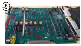
Next, remove the EPROM at location D2 (furthest to the left in the photo) and install your new freeplay chip. Detailed instructions on how to remove/install EPROMs can be found on page 2.
