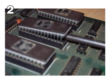
Next, slide the screwdriver forward towards the front of the EPROM and give it another twist so that more pins come out of the socket. When you twist, you want to make sure the screwdriver is pressing against the plastic bits of the socket and not the circuit board underneath the chip or you could damage your PCB.
