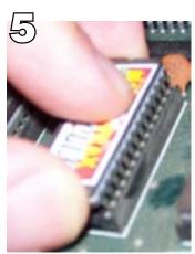
Next, bring the opposite row of pins down to line up with the other side of the socket. You may need to apply slight, even pressure to the chip to seat the pins into the socket. Do not apply full pressure until you're sure all the pins are lined up with the socket. Visually check for any pins that are not seated.
