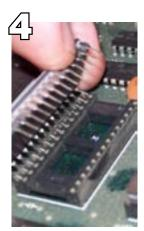
To install the new chip, first, make note of the notch at the top of the chip. This should face the same direction as the notches on the other EPROMs on the PCB. Then, line up the pins of one row with the socket. Don't apply any pressure at this point.
