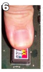
When you're sure all pins are properly aligned in the socket, apply firm, even pressure with your thumb in the center of the chip to press the pins fully into the socket. You should not have to force the chip. If you suspect you bent a pin, remove the chip, straighten the pin and try again.
