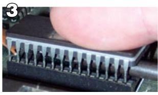
When the chip has lifted up enough that you can get the screwdriver all the way under, place your index finger over the chip, holding the screwdriver underneath with the rest of your fingers and gently lift the EPROM the rest of the way out of the socket. Store the EPROM in a safe, static-free place in case you ever need it.
